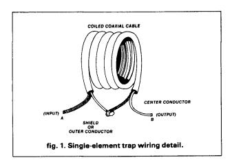
which is predictable, between the center conductor and shield. This capacitance can be employed in an LC network such as a tank circuit, which presents a high impedance at resonance.
