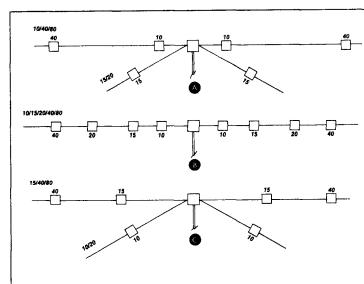
fig. 4. Trap antenna designs. Configuration in use by the author is a combination of horizontal trapped dipoles (A). Single dipole trapped antenna has narrow bandwidth (B). Recommended optimum multiband dipole is shown in C.
