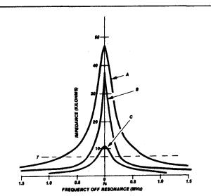
fig. 6. Comparison of relative rejection of 15-meter traps. A represents the single-element trap connected as described in the text. B represents the commercial trap of conventional design that was evaluated by the author. C represents the single-element trap's rejection if improperly connected as discussed in the text. Note the 7 kilohm bandwidth improvement over the conventional design. The rejection is plotted versus frequency away from resonance  $\{f_c\}$ .
