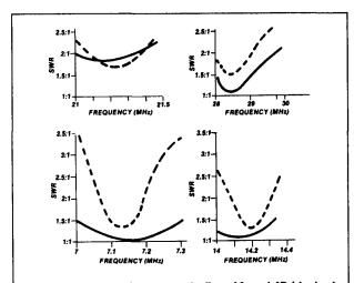
fig. 5. SWR plots of antennas in figs. 4A and 4B (dashed lines) illustrating effects of traps on antenna bandwidth.
